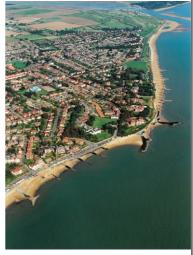
direction. The works at Cobbolds Point have created conditions which are more capable of retaining material under a range of conditions. However, this has also resulted in a readjustment of the material within the artificial bays created causing a draw down on beaches central to each bay against the back shore defences.
