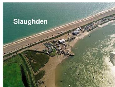
Within the estuary the seaward edge of the Slaughden Bend is protected by the various quays and slipways, and the nearshore slope is quite shallow. There are major flood embankments to the main flood compartments.
