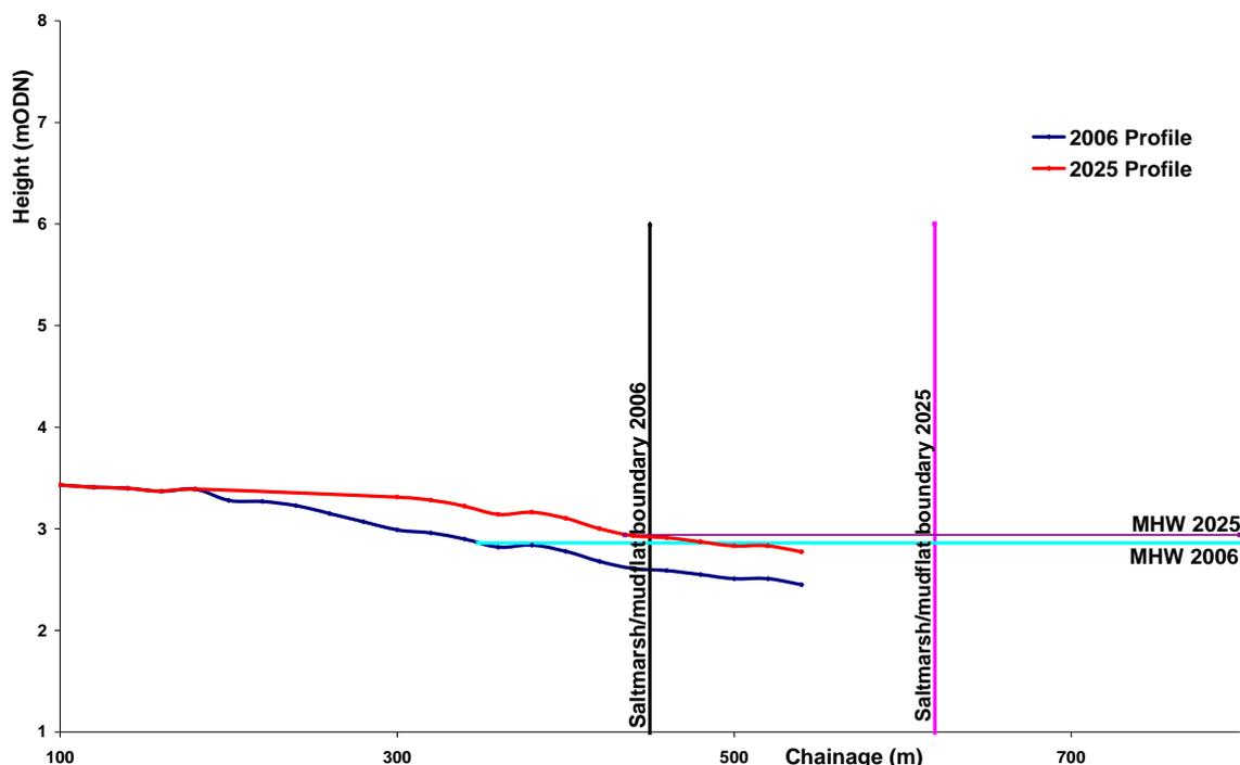
Figure F3.5.5 is also important as it suggests that coastal squeeze is not occurring to the same extent as on frontages A and B. This is mainly due to the fact that along frontage D (and C) there has not been the degree of reclamation as along frontages A and B, where land claim has encroached too far onto the former mudflat. Therefore the saltmarsh/mudflat system exists under a more natural state and follows a more natural profile.
