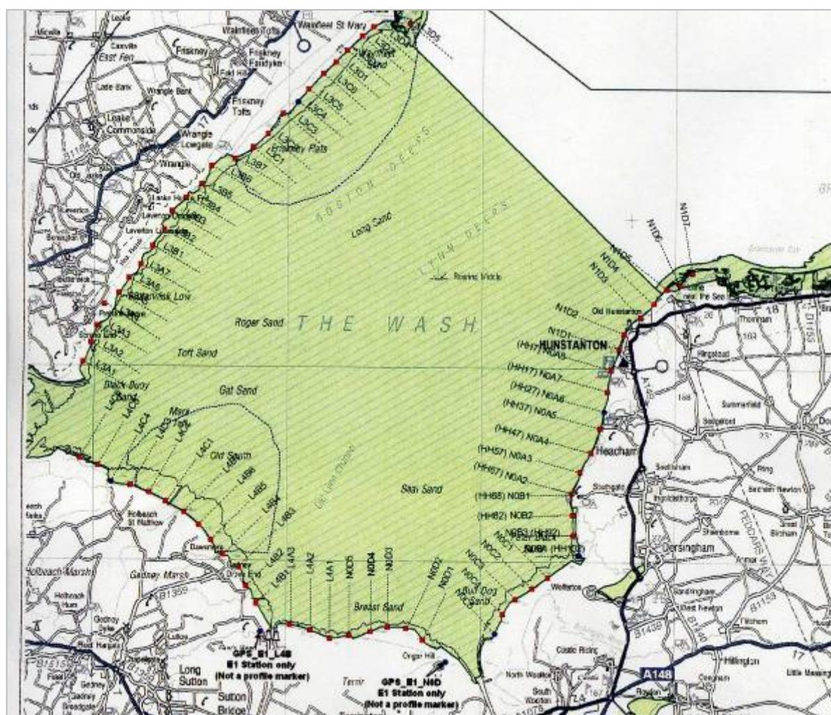
Cross sections have been taken from SAR ground level data and compared with the local survey data. These cross sections can be seen in figure F6.14 to figure F6.19. These show that there is extensive salt marsh width, typically 800m (300-1500m) in front of the earth embankments, currently advancing on average 1m/year. The earth embankments have crest heights between 6.1 and 7.2mODN. The salt marsh height varies around MHWS at 3.7mODN.
